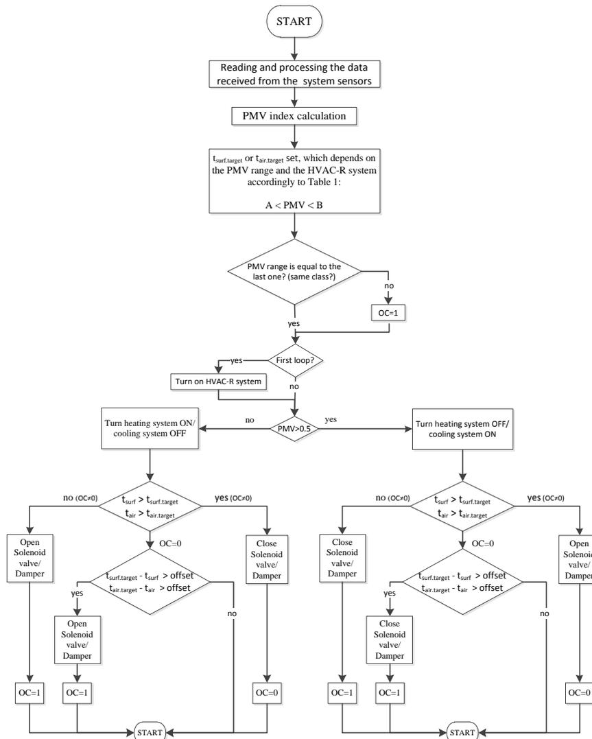
**Fig. 1 - Flowchart of the controller program based on the PMV index.**
