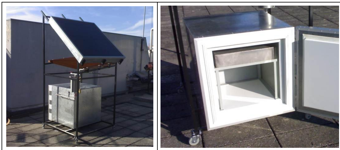
Figure 3 – Pictures of the solar adsorption refrigerator and the placement of the evaporator inside the refrigerated cabinet.
